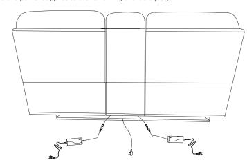
① Make sure all plugs are connected on the product before plugging the power cords into a wall outlet - otherwise product damage may occur. The USB ports (where applicable) are designed with working voltage of 5V and can NOT be used to supply power for laptop computers (neither PC or Mac). Plugging a laptop computer to the USB port may end up damaging either the computer or the USB port due to unmatched working voltage.
