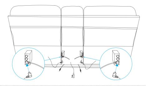
Step 3 Connect the two power supplies to the remaining available plugs.
